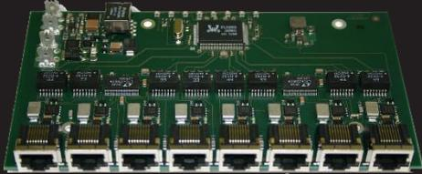
8x 1GbE RJ-45 Ethernet NTP & ITPP EEE1588 (software timestamping)
