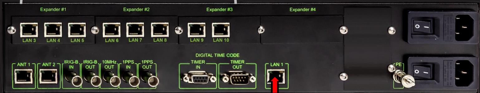
LAN interfaces can be numbered 1-10 or in 2 groups numbering 1-2 (compatibility mode) 1-8 extension floor
