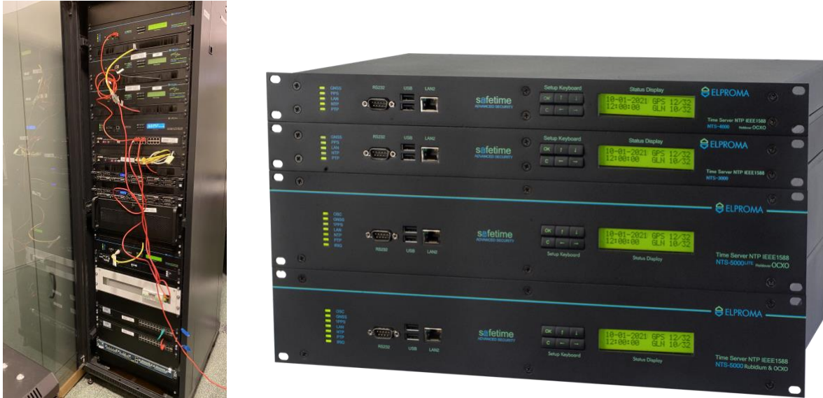
Fig. 24. "Clepsydra " Time Synchronization System Node at the Polish Air Navigation Services Agency (PANSa), a Part of the Distributed Synchronization Architecture Possessed by PANSa in an Intercity Convergence Setup. The Presented Node Contains 5x NTS-5000 Class Servers, Including One Atomic Server linked to Cesium Atomic Clock.
