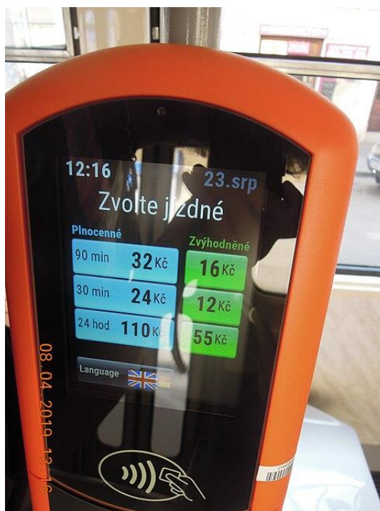
Rys. 18. GPS Week Number Rollover Error from 2019 on Being aircraft gyroscope (left side) and TAX telemetry system in Prague in Czechia. Source: self-produced
