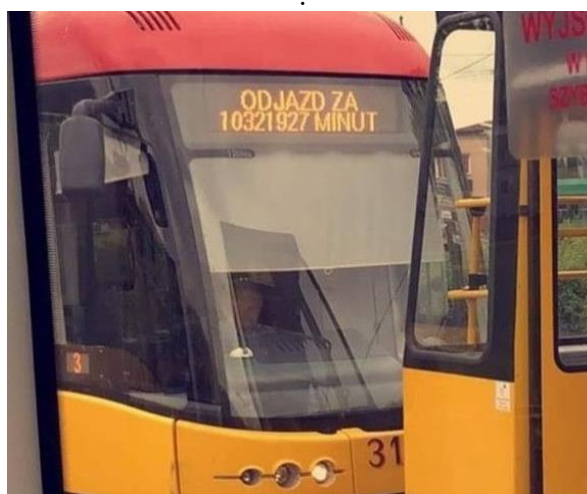
Fig. 17. GPS Week Number Rollover Error from 2019 on Tramways in Warsaw Poland. Source: self-produced
