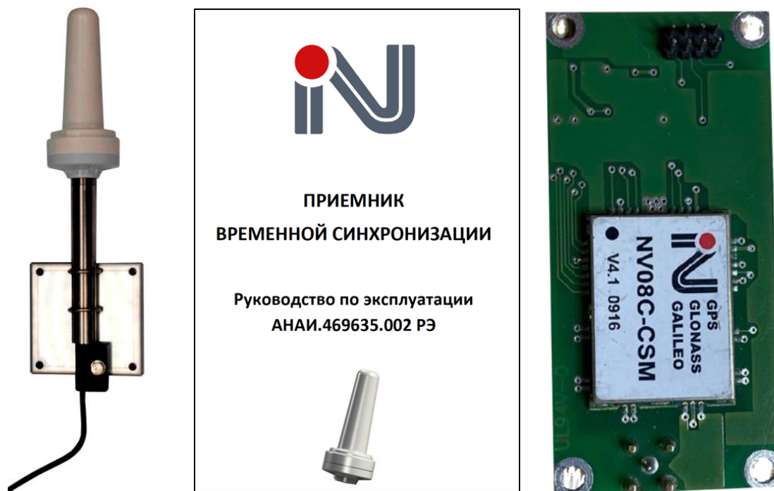
Fig. 12. The Russian Receiver NVS ANAI 469635.002 (on the left). It based on the GLONASS System as Primary and Its Internal NV08C-CSM (on the right) Chipset Sold Commercially Under the Swiss Brand NVS and Exported Globally.
