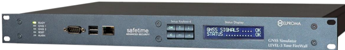
Fig. 26. Front Panel View of the Elproma LEVEL-3 GNSS Simulator. This Network GNSS Simulator Receives Information from Remote NTP/PTP Servers at GUM RP (eCzasPL) and Converts it into a Simulated Antenna Signal for the NTS-5000 Time Server.
