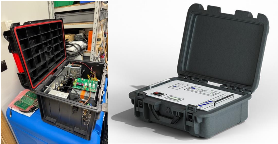
Fig. 41. Polish portable UTC "defibrillator" ELPROMA, on the right Israeli "Time Loader." The size of the device determines the UTC support time and depends on the battery capacity. Source: Elproma
