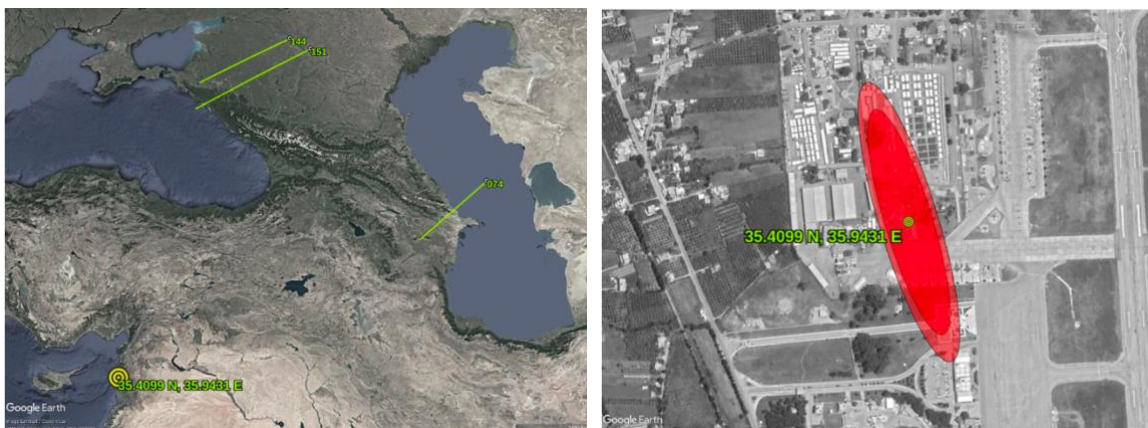
Fig. 21. Calculations based on Doppler history indicated that a transmitter in a Russian military base in Syria was responsible for GPS interference in the Black Sea region.
