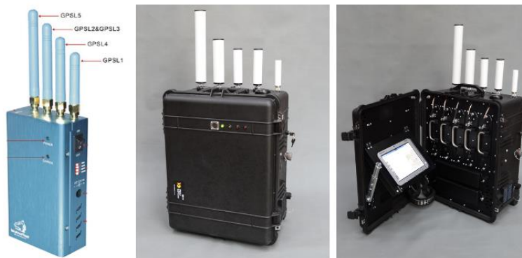
Fig. 34. Chinese-made mobile GPS jammer (on the left). Polish-made PIAP and iTTi/Łukasiewicz professional programmable jammer (right side), model ZKR-1 with 150W power and a frequency range of 25-5800 MHz, capable of generating continuous and responsive jamming.
