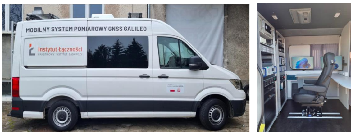
Fig. 35. Mobile measurement station for testing the quality and jamming of GNSS signals Source: Institute of Telecommunications
