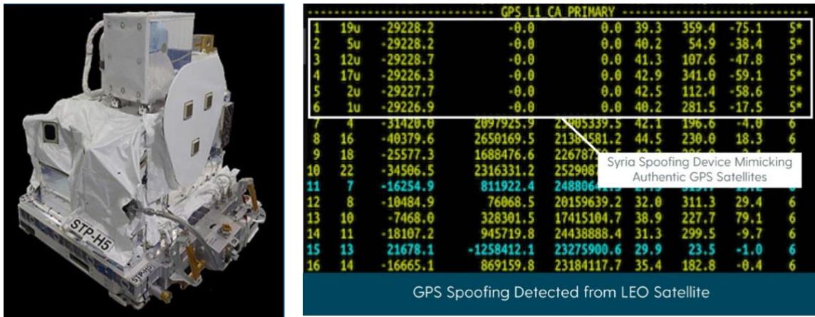
Fig. 18. STP-H5 sensor, installed on the International Space Station (ISS) at an orbit of approximately 400 km above Earth, is equipped with a GPS receiver designed for ionospheric research. Decoded data revealed a value of 0 in the LNAV fields, indicating the presence of "coded jamming."
