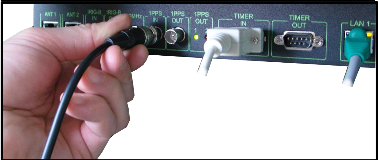
Connecting PPS (BNC) and ToD RS232 cables to NTS (the NTS-x000 back panel view)
