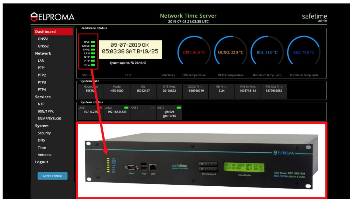
6x LED indicators (from left: OSC, GNSS, PPS, LAN, NTP, PTP, IRIG)
