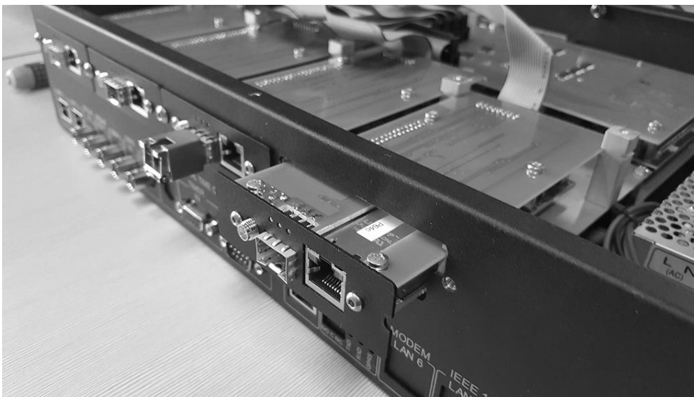
PTP1-PTP4 hardware extension cards at NTS-5000 (front view)
