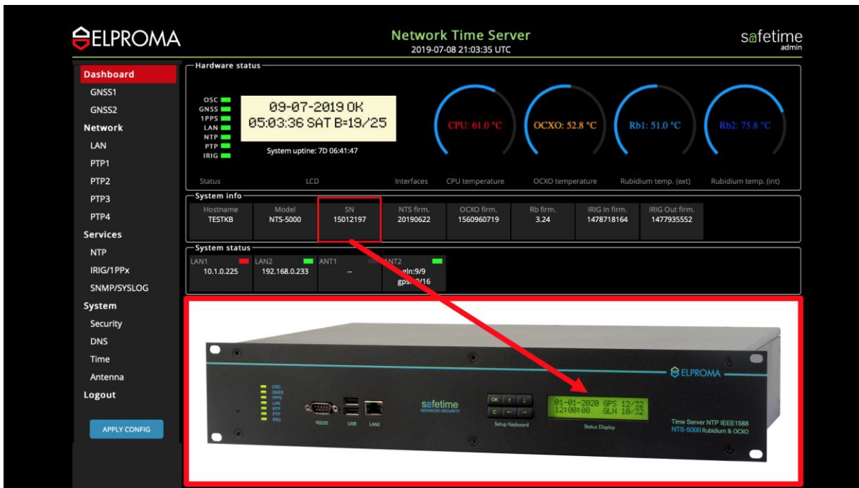
Serial number available on LCD after power-on. Also located on the back-panel S/N sticker
