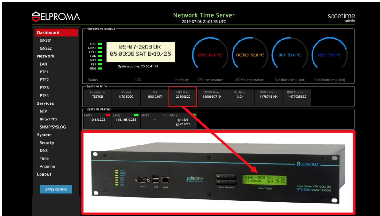
Firmware serial available on LCD after power-on. Also available as KEYBOARD command sequence
