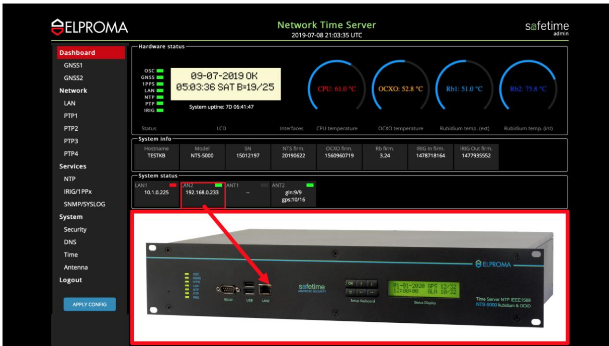
IPv4 address & LAN2 front panel LED indicator (flash green when Ethernet network cable connected)
