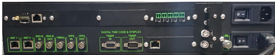
NTS-TC (time-converter PTP-2-IRIG) – back panel view (max. version w/ 4x RS422, 2x FO, 2x BNC TTL 5V AM/DCLS)
